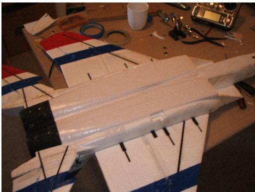
As the model is a hand launch and belly landed a layer of white gaff tape is used to give an easy clean smooth surface to the bottom of the model. It also acts to cover up the scar this operation caused.
