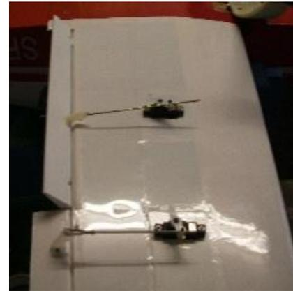
plywood plate are glued using CA. Hopefully you can also make out the 45 degree chamfer for the flap. Wayne did the chamfer in one single movement. All I did was hold the wing steady, very impressive. The theory to the chamfer is to allow a 90 degree flap action if you so desire. Unfortunately my initial setup couldn't, as I didn't have any ball-link control rod ends with me.
