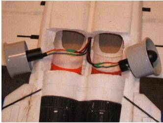
Measuring to make sure the surgical cuts were either side of the EDF units a very sharp hobby knife was used to cut out the bottom as shown. Note the cross cuts are square and the side cuts are on an angle. This is to assist in stitching up the patient after surgery.
