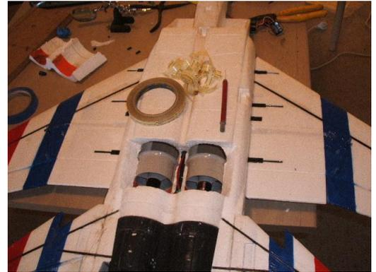
Now it's time to stitch up the wound. Using double sided tape again on the outer angled cuts the opening is closed.
