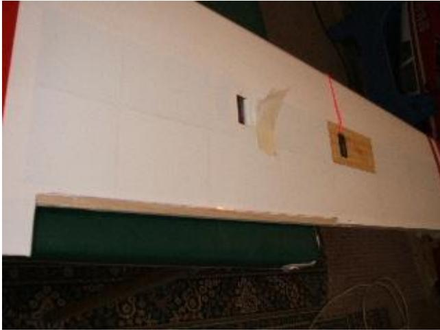
In the picture to the left you can see the wing is prepared, new servo mount glued using 5 minute epoxy and the balsa rails to hold the
