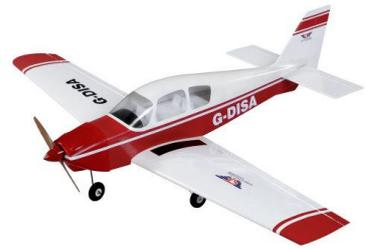
These days ARF's go together pretty quick and the quality of finish has come a long way, especially for these budget conscious Chinese kits. This particular ARF is ply and balsa for the lower half of the fuselage and moulded ABS plastic for the cabin half. Pretty clever, if you ask me.
